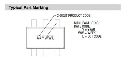
The form of the part numbers made at the new additional manufacturing site will change because of a small change in the part marking for trace-ability purposes. The quality, reliability and performance of the overvoltage protectors produced at the new manufacturing site will be the same as those from the existing plant. The production lead times of these overvoltage protectors should improve gradually as our capacity is expanded. The country of origin will remain the same.
