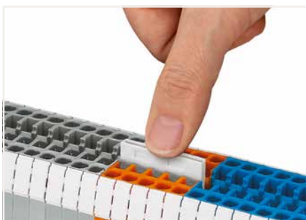
Push jumper bars down firmly until fully inserted. When using multipole bars, push alternately on the right and then left side until installed. Push-in type jumper bars 1-3-5-7 or 1-4-7 are available upon request.
