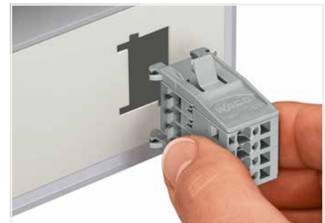
Insert a male connector with snap-in flanges (769-604/005-000) into the cutout.
