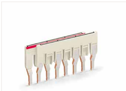
Staggering jumpers in a single jumper slot. Custom staggered jumpers can be created, e.g., for bridging over a terminal block with a different potential. Make sure that only one contact lug is in contact with the terminal block.
