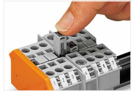
Commoning terminal blocks of different sizes – step down. Push down the step-down jumper until fully inserted.
