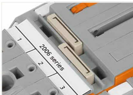
Commoning a 15 mm-wide terminal block via push-in type jumper bars: 1 to 3 (2006-433) and 1 to 5 (2006-435).
