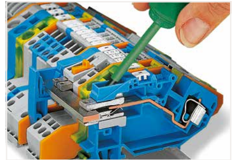
Operating an N-disconnect slide link.
