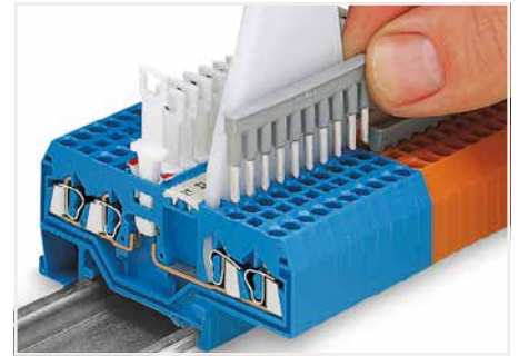
Commoning front-entry disconnect terminal blocks via comb-style jumper bar using a 10-pole operating tool.
