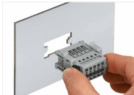
Insert a male connector with snap-in flanges (769-605/006-000) into the cutout.
