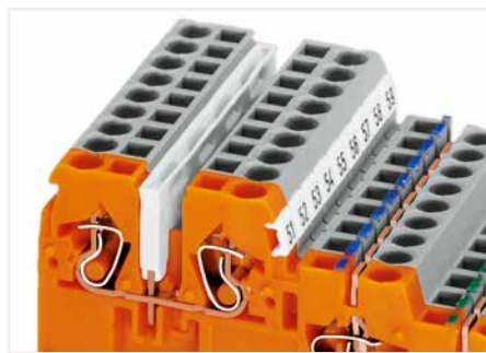
Commoning signal level voltage via insulated push-in type jumper bars (870 Series) – 2- to 9-way, depending on application. Sensor LED terminal blocks cannot be commoned!
