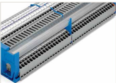
The compact busbar carrier (1.5 mm thick), which is placed every 200 mm, provides additional busbar support for longer assemblies.
