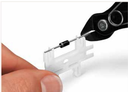
Cutting component to the proper length.
