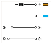
Sensor LED terminal block; for fuse plugs; for PNP (high-side) switching sensors; without end plate
