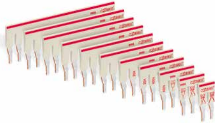
Staggered jumper (seven contacts): Individual jumper contacts can be broken off by bending them. The remaining piece of insulation will meet requirements for clearances and creepage distances.
