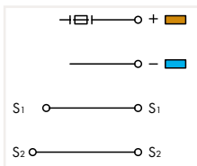
Sensor LED terminal block; for fuse plugs; for PNP (high-side) switching sensors; with gray end plate Terminal block width: 6 mm / 0.236 inch
