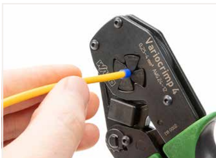
Squeeze handles until ratchet mechanism is released.
