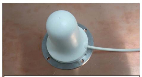
Antenna mounted on a Metal surface (example)
