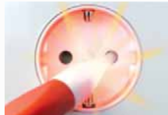
The testing pen detects the phase and neutral conductor
