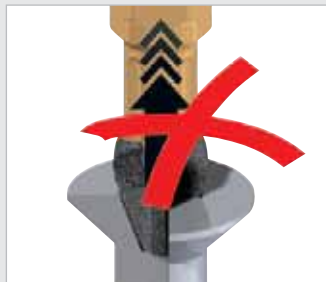
The Dura coating reduces CamOut effects to an unbeatable minimum - no more slipping out of the bit from the screw head.
