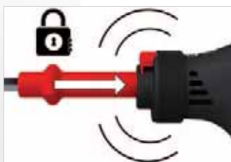
Automatic / mechanical blade locking
