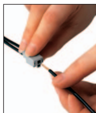
Solid conductor strip (8–9 mm) and connect conductor
