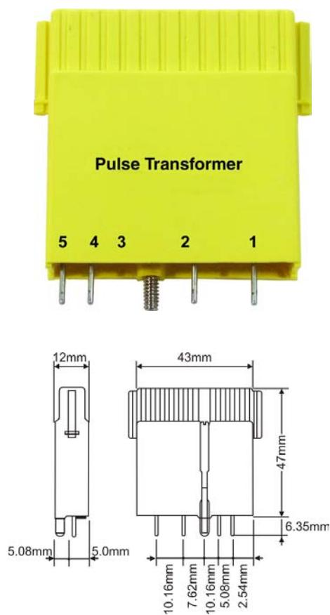
Pulse transformer technology for isolating I/O signals offers significant advantages over optical isolation and electromechanical relays. Most notably, pulse transformer I/O modules provide higher transient immunity, and high input-to-output isolation.
