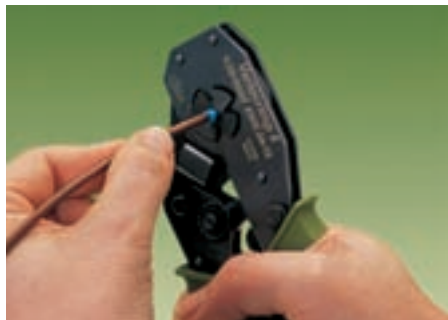
Introduce conductor with ferrule into crimping station. Squeeze handles until ratchet mechanism is released.
