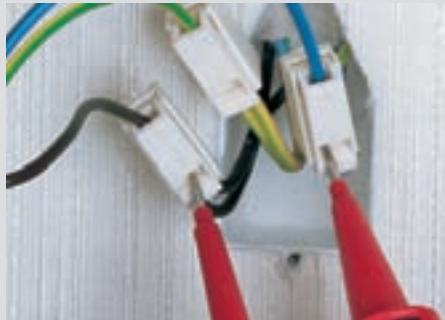
Testing through separate test slot
