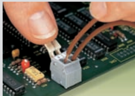
Connection/removal of conductors, series 255 Finger operation Terminal strips with finger operated levers see General Catalogue
