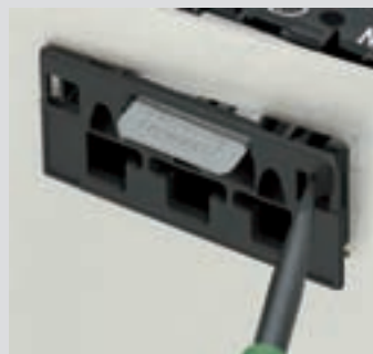
Remove the snap-in type connector from outside the enclosure inserting a screwdriver from the front
