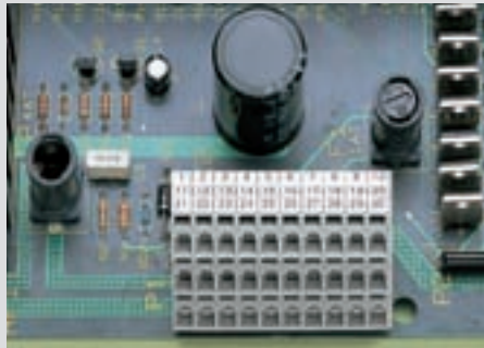
Space saving with triple deck terminal strip
