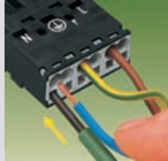
Open clamping unit using a screwdriver (2.5 x 0.4) mm and insert stripped wire as far as possible
