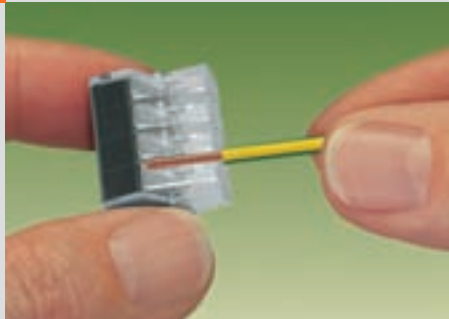
Strip solid conductor to 12 mm / 0.47 in
