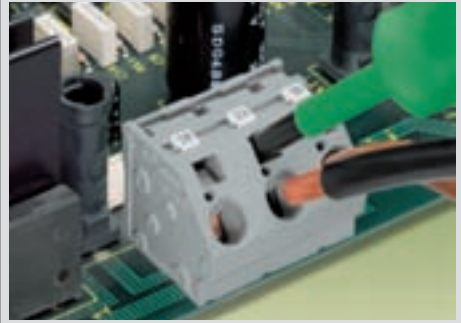
Connection of conductors using screwdriver 5.5 mm
