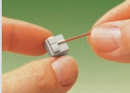
Strip solid conductor to 5 – 6 mm / 0.22 in
