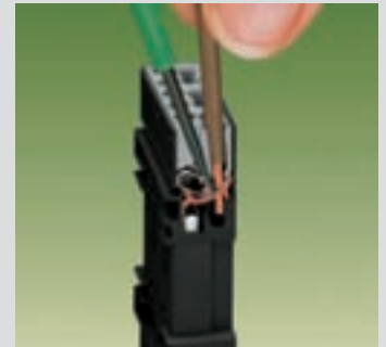
Open clamping unit using a screwdriver (2.5 x 0.4) mm and insert stripped wire as far as possible
