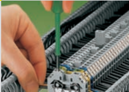
Open the clamping spring using a 2.5 mm screwdriver and insert the conductor as far as possible
