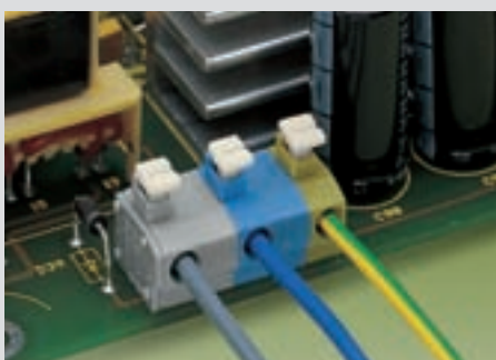
Example of application – terminal strip for field connections
