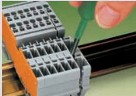
Unlock assembly with screwdriver (3.5 x 0.5 mm) and remove terminal block via release lever
