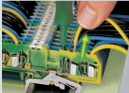
Wire removing with screwdriver
