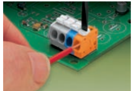
Connection/removal of fine-stranded wires: Open the clamping unit using push button and fully insert stripped wire into the terminal block
