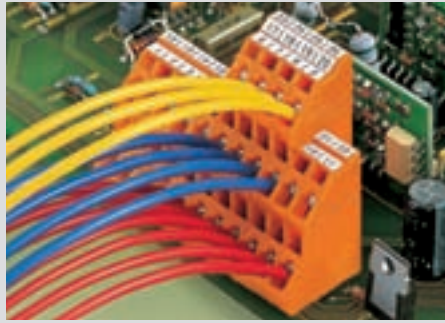
Mix of double deck and triple deck terminal strips
