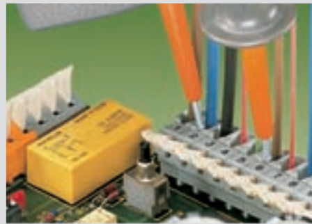
Testing with test probes
