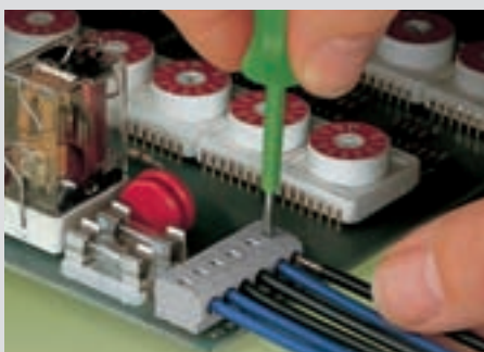
Removal of conductors without push button
