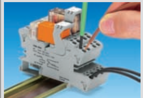
Solid conductors or flexible conductors with ultrasonically bonded wire ends or ferrules can be simply pushed in - without using a screwdriver
