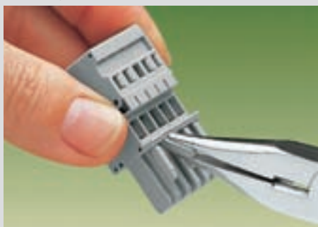
Coding a female plug - removal of coding finger(s). Do not break off the first and last latch position coding finger!
