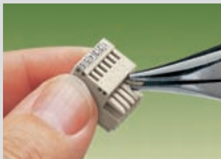
Coding of a female connector – removal of coding finger(s)
