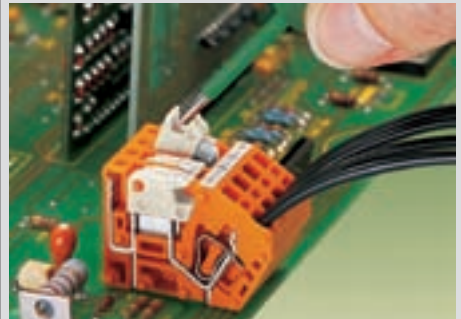
Opening of disconnect
