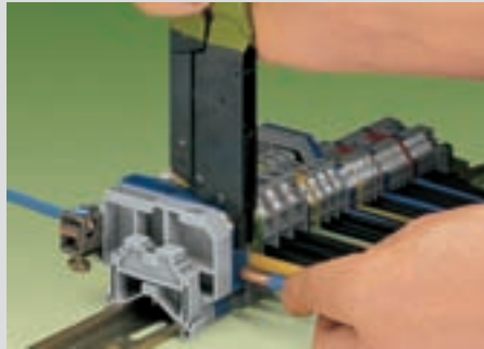
The plunger is placed into the upper operating slot of the side-entry terminal block and the clamp is hooked into the lateral operating hole. The contact is fully opened by pressing the handles together until they engage. Insert the conductor as far as possible.
