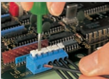
Fine-stranded wire, tip bonded Connection/removal using push button
