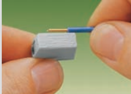
Strip conductor to 9 – 11 mm / 0.39 in
