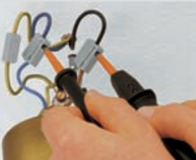
Testing through separate test slot
