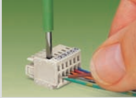
Connection of conductors – side-entry wiring – with screwdriver (2.5 x 0.4) mm
