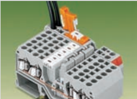
Staggered jumper for sophisticated wiring jobs. Push jumpers down FIRMLY until FULLY inserted
