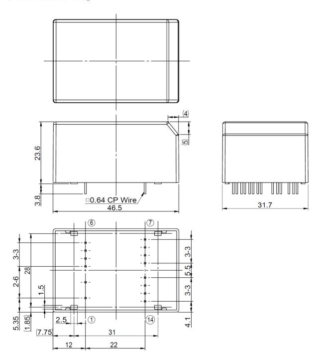
Note :1.The dimensional tolerance without directions is  $\pm$  0.5mm.
