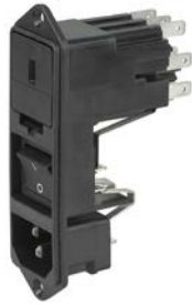
IEC connector C14 with fuse holder 1- or 2-pole with voltage selector and line switch 2-pole Screw-on version from front or rear side Order required accessories separately
