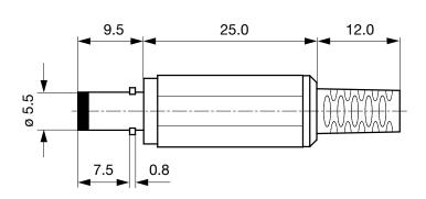
Cable diameter max. 4.0 mm
