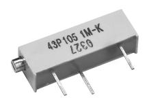
The Model 43 is manufactured to the highest international standards. This product, sealed to 85°C for 1 minute (IEC. 68-2-17) has an effective travel of 20 turns nominal and a resistance range of  $10\Omega$  to  $2M\Omega$ .
