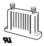
The Model 183 external multiplier enables an iron-vane type voltage meter to monitor up to 1000 AC volts. An external multiplier is used with a 150 AC voltage meter that is scaled proportionally to your measurement range. Simpson's AC meters having a range of 500 volts or higher are furnished with the Model 183. Simpson's external multipliers are available for immediate delivery from your local distributor. Other intermediate ranges are available on special order.
