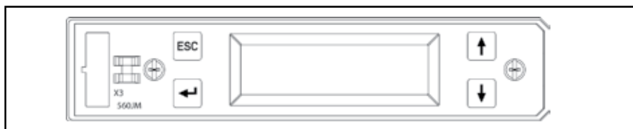
Model 576 Electronic Trip Unit has an LCD display
