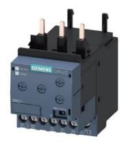
Monitoring relay, can be mounted to Contactor 3RT2, Size S0 basic, analog adjustment Apparent current monitoring 4...40 A, 50...60 Hz, 2-phase Supply 24 V AC/DC 1 change-over contact Monitoring for Current overshoot and undershoot Phase failure, Cable break with or without fault buffer ON delay 0-60 s Noise pulse suppression 0-30 s Switching hysteresis 6% Screw connection system
