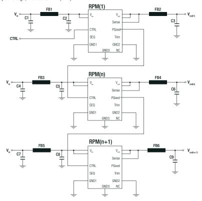
To sequence multiple converters to start at the same time (set output voltage is reached at the same time), the following schematic may be used:
