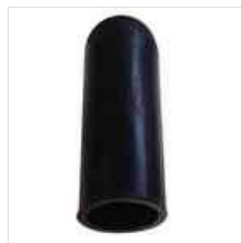
Masking Straight Cap & Plug: .172 in (4.4 mm) Cap ID, 180 °C (356 °F) Max. Temp.,.500 in (12.7 mm) Height
