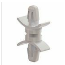
PCB Sprt, Top HI: Lock Arrow .125 in/ .030 in-.078 in Pnl, Bottom HI: Lock Arrow .125 in/.030 in-.078 in, Nat, UL94 V-2 Nylon 6/6
