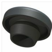
Body Plug: .394 in (10 mm) Panel Hole Size, .032 - .079 in (0.8 - 2 mm) Panel Thickness
