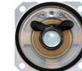
AS05008MS-R 12 H x 50.5 W x 50.5 L Frequency range: 0.80-7.0kHz Max input: 3 W Rated input: 1.5 W
