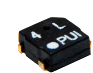
SMT-0540-T-7-R 2 H x 5 W x 5 L Frequency: 4,000 ± 500Hz Voltage range: 2 – 4 Vp-p
