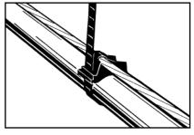
Support tie shown when properly installed. If releasability is not required, tip can be cut off.
