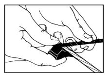
Snap groove portion of tie onto support strand.
