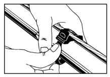
Position cable against tie spacer and thread tail through slot in head. Push upwards on body of tie until snug.
