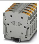
High-current terminal block, nom. voltage: 1000 V AC / 1500 V DC, nominal current: 150 A, connection method: Power-Turn connection, number of connections: 2, number of positions: 1, cross section: 10 mm² - 70 mm², AWG: 8 - 2/0, width: 20 mm, color: gray, mounting type: NS 35/15
