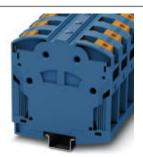
High-current terminal block, nom. voltage: 1500 V DC / 1000 V AC, nominal current: 309 A, connection method: Power-Turn connection, number of connections: 2, number of positions: 1, cross section: 50 mm² - 150 mm², AWG: 1/0 - 300 kcmil, width: 31 mm, color: blue, mounting type: NS 35/15
