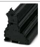
Fuse modular terminal block, fuse type: Glass / ceramics / ..., connection method: Screw connection, cross section:  $0.14 \text{ mm}^2$ -  $4 \text{ mm}^2$ , AWG: 26 - 10, nominal current: 30 A, nom. voltage: 500 V, width: 6.2 mm, fuse type:  $6 \text{ J} \times 20$ , mounting type: NS 35/7,5, NS 35/15, color: black
