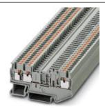
Disconnect terminal block, nom. voltage: 400 V, nominal current: 20 A, connection method: Push-in connection, cross section: 0.14 mm² - 4 mm², AWG: 26 - 12, length: 74 mm, width: 5.2 mm, color: gray, mounting: NS 35/7,5, NS 35/15, nom. voltage: 400 V
