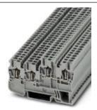
Sensor/actuator terminal block, nom. voltage: 250 V, nominal current: 18 A, connection method: Spring-cage connection, number of connections: 4, cross section: 0.08 mm² - 4 mm², AWG: 28 - 12, width: 5.2 mm, color: gray, mounting type: NS 35/7,5, NS 35/15
