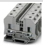
Bolt connection terminal block, Connection type: Bolt connection, Cross section: 2.5 mm² - 35 mm², AWG: 14 - 2, Nominal current: 125 A, Nominal voltage: 1000 V, Length: 84 mm, Width: 20.3 mm, Color: gray, Assembly: NS 35/7,5, NS 35/15
