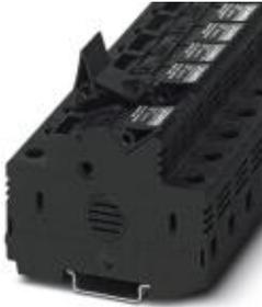
Fuse modular terminal block, Connection method: Screw connection, Cross section: 1.5 mm<sup>2</sup>- 25 mm<sup>2</sup>, AWG: 16 - 4, Nominal current: 32 A, Nominal voltage: 690 V, Width: 18 mm, Fuse type: Midget / 10.3 x 38, Fuse type: Glass, Mounting type: NS 35/7,5, NS 35/15, Color: black
