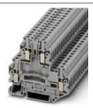
Disconnect terminal block, connection method: Screw connection, cross section: 0.14 mm² - 6 mm², AWG: 26 - 10, width: 6.2 mm, color: gray, mounting type: NS 35/7,5, NS 35/15
