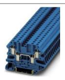
Feed-through terminal block, nom. voltage: 500 V, nominal current: 32 A, connection method: Screw connection, number of connections: 4, cross section:0.14 mm² - 6 mm², AWG: 26 - 10, width: 6.2 mm, height: 46.9 mm, color: blue, mounting type: NS 35/7,5, NS 35/15
