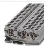
Feed-through terminal block, Connection method: Spring-cage connection, Cross section: 0.2 mm<sup>2</sup> - 10 mm<sup>2</sup>, AWG: 24 - 8, Width: 8.2 mm, Color: blue, Mounting type: NS 35/7,5, NS 35/15
