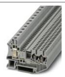
Feed-through terminal block, Connection method: Screw connection, Cross section: 0.5 mm<sup>2</sup> - 16 mm<sup>2</sup>, AWG: 20 - 6, Width: 10.3 mm, Color: gray, Mounting type: NS 35/7,5, NS 35/15
