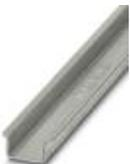
DIN rail, unperforated, Standard profile 2.3 mm, width: 35 mm, height: 15 mm, acc. to EN 60715, material: Steel, galvanized, passivated with a thick layer, length: 2000 mm, color: silver
