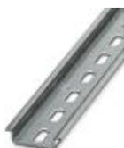
DIN rail perforated, Standard profile, width: 35 mm, height: 7.5 mm, acc. to EN 60715, material: Steel, galvanized, length: 2000 mm, color: silver
