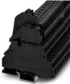
Fuse modular terminal block, fuse type: Glass / ceramics / ..., connection method: Screw connection, cross section: 0.2 mm<sup>2</sup>- 4 mm<sup>2</sup>, AWG: 24 - 12, nominal current: 32 A, nom. voltage: 24 V, width: 8.2 mm, fuse type: G / 5 x 20, mounting type: NS 35/7,5, NS 35/15, NS 32, color: black
