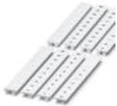
Zack marker strip, Strip, white, labeled, can be labeled with: CMS-P1-PLOTTER, printed horizontally: consecutive numbers 1 ... 10, 11 ... 20, etc. up to 491 ... 500, mounting type: snap into tall marker groove, for terminal block width: 8.2 mm, lettering field size: 10.5 x 8.15 mm, Number of individual labels: 10
