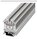
Feed-through terminal block, Connection method: Screw connection, Cross section: 0.2 mm<sup>2</sup> - 4 mm<sup>2</sup>, AWG: 24 - 12, Width: 5.2 mm, Color: gray, Mounting type: NS 32, NS 35/15, NS 35/7,5
