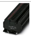
Flat-type fuse terminal block, cross section: 0.2-6 mm², AWG: 26-8, width: 8.2 mm, color: black, with LED, voltage LED: 60 V DC, current LED: 2 mA
