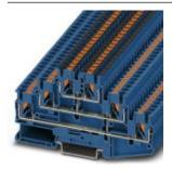
Multi-level terminal block, With equipotential bonder, nom. voltage: 500 V, nominal current: 20 A, connection method: Push-in connection, number of connections: 6, cross section: 0.14 mm² - 4 mm², AWG: 26 - 12, width: 5.2 mm, height: 56.5 mm, color: blue, mounting type: NS 35/7,5, NS 35/15
