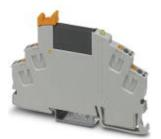
Pre-assembled solid-state relay module with push-in connection, consisting of: relay base with ejector and plug-in miniature solid-state relay. Input voltage: 24 V DC. Output: 3 - 33 V DC/3 A
