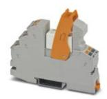
Pre-assembled relay module with push-in connection, consisting of: relay base, power contact relay, plug-in display/suppressor module, and retaining bracket. Contact type: 1 PDT. Input voltage: 24 V AC
