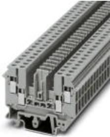
Disconnect terminal block, Connection type: Screw connection, Cross section: 0.2 mm<sup>2</sup> - 6 mm<sup>2</sup>, AWG: 24 - 10, Nominal current: 16 A, Nominal voltage: 400 V, Length: 63.5 mm, Width: 6.2 mm, Color: gray, Assembly: NS 35/7,5, NS 35/15, NS 32
