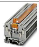
Knife disconnect terminal block, With test socket screws for insertion of test plugs, Connection type: Screw connection, Cross section: 0.2 mm² - 6 mm², AWG: 24 - 10, Nominal current: 16 A, Nominal voltage: 630 V, Length: 63.5 mm, Width: 6.2 mm, Color: gray, Assembly: NS 35/7,5, NS 35/15, NS 32
