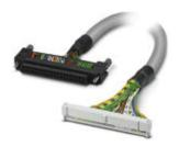
Round cable set; controller: Siemens S7-300 (6ES7 322-1BP00-0AA0 and 6ES7 322-1BP50-0AA0 (negative switching)); connection 1: Fujitsu connector (1x 40-position); connection 2: IDC/FLK socket strip (1x 50-position); cable length: 2 m
