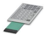
Membrane keypad, self-adhesive, silver conduction technology, 45 keys, embossed, 4 colors, connection cable: 77 mm, with crimp female connector RM 2.54 mm, operating temperature -20 °C ... 70 °C
