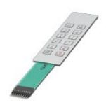
Membrane keypad, self-adhesive, silver conduction technology, 12 keys, embossed, 3 colors, connection cable: 88.5 mm, with crimp female connector RM 2.54 mm, operating temperature -20 °C ... 70 °C
