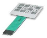
Membrane keypad, self-adhesive, silver conduction technology, 12 keys, embossed, 3 colors, connection cable: 100.5 mm, with crimp female connector RM 2.54 mm, operating temperature -20 °C ... 70 °C
