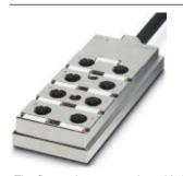
Sensor/actuator box, application: Standard, connection method: M12 socket Metal, number of slots: 4, number of positions: 5, coding: A - standard, slot assignment: Double, status display: No, Universal; master cable connection: Fixed connection 180°, PUR/PVC, cable length: 5 m, shielding: yes
