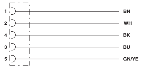
Contact assignment of the M12 sockets
