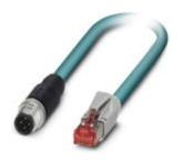
Assembled Ethernet cable, CAT5e, shielded, 2-pair, AWG 26 stranded (7-wire), RAL 5021 (water blue), M12 4-pos. D-coded on RJ45 connector, length: 2 m, customer version
