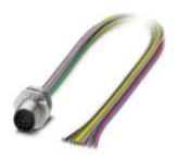
Sensor/actuator flush-type plug, 12-pos., M12 SPEEDCON, front/screw mounting with M16 thread, with 0.5 m PVC litz wire, 12 x 0.14 mm<sup>2</sup>
