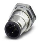
Bus system flush-type plug, 4-pos., M12 SPEEDCON, D-coded, rear/screw mounting with M12 thread, with straight solder connection
