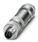
Connector, Universal, 4-position, shielded, Plug straight M8, Screw connection, knurl material: Nickel-plated brass, external cable diameter 3.5 mm ... 5.5 mm
