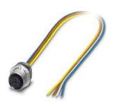
Bus system flush-type socket, PROFINET, 4-pos., M12-SPEEDCON, D-coded, front/screw mounting with M16 thread, with 0.5 m TPE litz wire, 4 x 0.34 mm<sup>2</sup>
